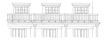
A row of columns supporting an entablature, and sometimes a pediment too, were often used to link the facades of a number of adjoining houses, or even an entire terrace of Georgian houses.
