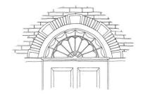
This arch window is an example of what could typically be found above a Georgian door, with panes of glass separated by tracery radiating out
